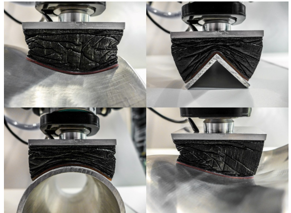
Flexible 3D fiber placement with FPP
